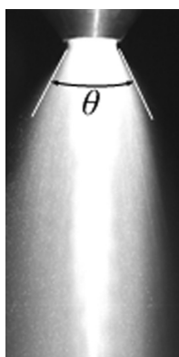
Figure 16. Schematic diagram of the dispersion angle (100 superimposed images, \Delta t = 0.001 s).
